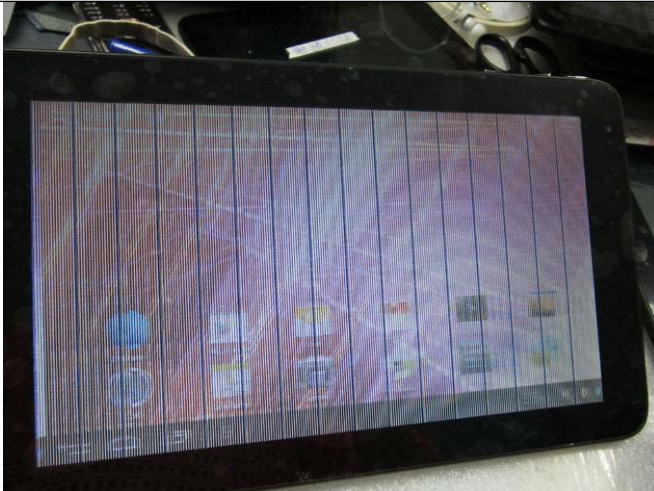
Screen flash /Unit dead when tear up the touch screen protective film
