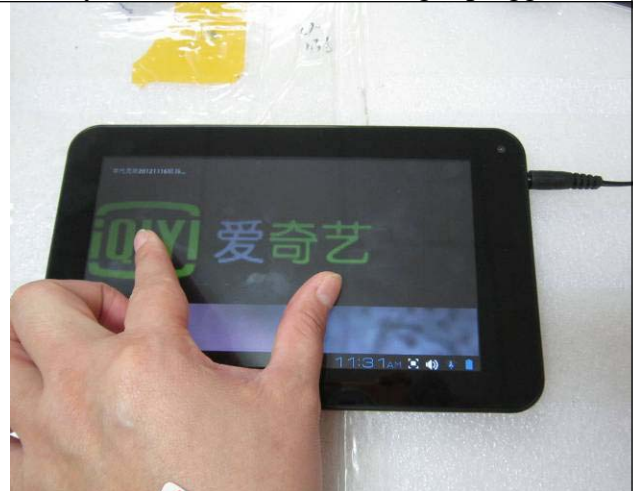
Touchscreen typing tested and used when battery is below 30% - Charger plugged in
