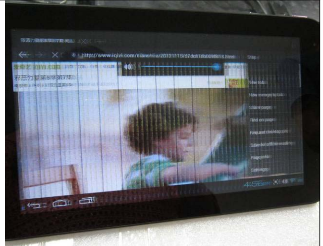
Screen flash /Unit dead when tear up the touch screen protective film
