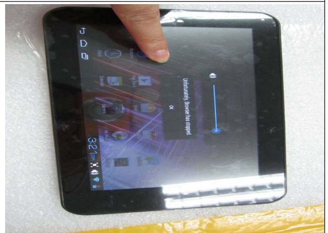
Sometimes touch screen malfunction
