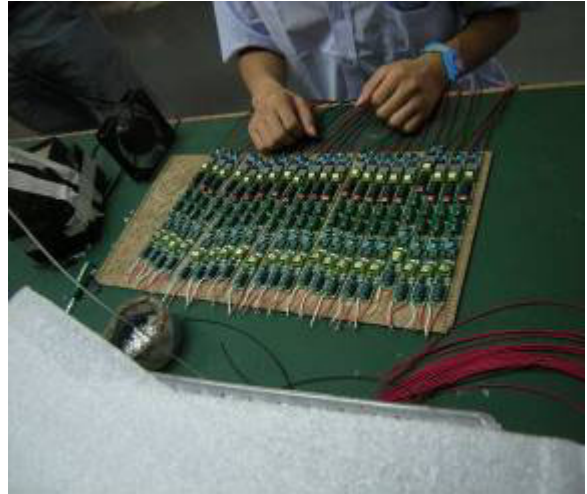
Welding for tube light manufacture
