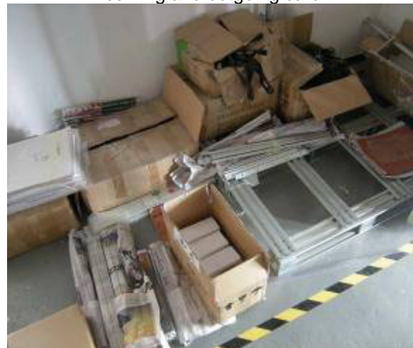
Non-conforming raw materials adequately segregated, but not Identified and labeled
